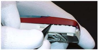
Turn around the phone release the other side from A-Cover. To avoid damages, plastic tweezers should be preferred. Where the clips are located can be seen in the right picture.
