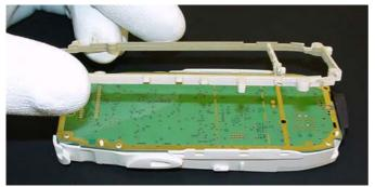
After removing the Spacer Frame, the CMT module is accessible.
