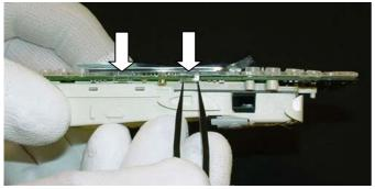
There are 3 clear plastic clips to release, which hold the Light Guide onto the UI module MU4. Two clips are on this shown side in the picture and one at the backside in the near of the speaker.
