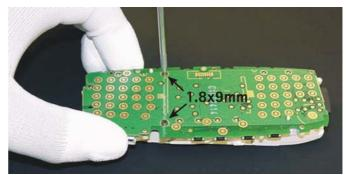
To remove the UI module MU4, 2 further screws have to be opened.
