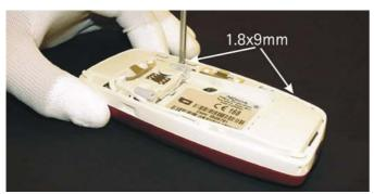
Before opening the unit the display should be protected with a foil. Then open the 2 upper screws from the B-Cover. Please note, that the unit has 16 screws which aren't equal in length and thread.
