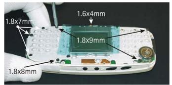
Unscrew the 8 screws from the Light Guide of UI module.
