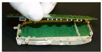
Lift up now the UI module and avoid touching the connector pads and keypad pads. The best way is, to use gloves.
