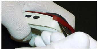
The A-Cover can be released from the lower right side on. Place the plastic tweezers between the cover clip and the power button. Same has to be done at the left side just near the Port Cover.
