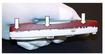
The cover is fixed with 3 plastic clips, which have to be released carefully. After that the cover can be removed together with the keymats.
