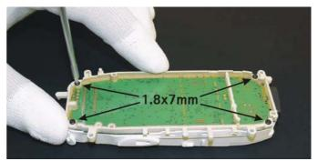
The Spacer Frame is fixed with 4 screws of the same size.
